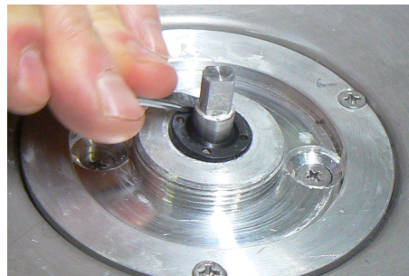
Place the new oil seal using the flat end of a screwdriver to fix it perfectly
