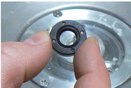
Take a new oil seal Paying attention to the orientation
