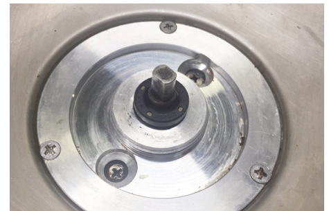
Position the second oil seal. Paying attention to the orientation
