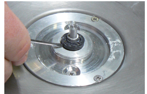
Raise the oil seal to be replaced with a screwdriver
